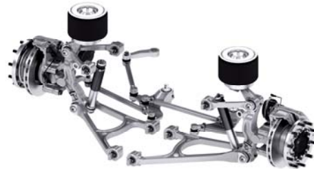
Fig. 2. Articulated front axle [2]
