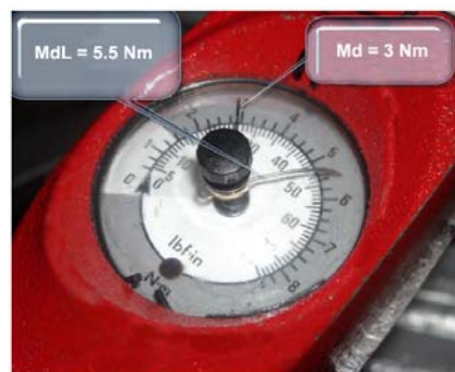
Fig. 5. Measurement of rotation moment using torque wrench [7]
